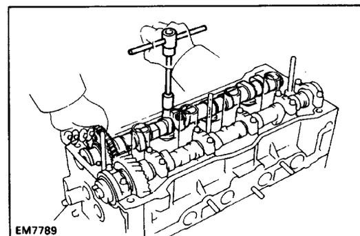
HINT: If the camshaft is not being lifted out straight and level, reinstall the bearing cap with the two bolts.
