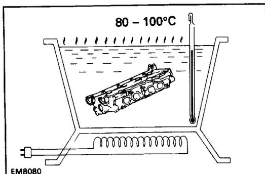
(f) Gradually heat the cylinder head to 80-100°C (176-212°F).
