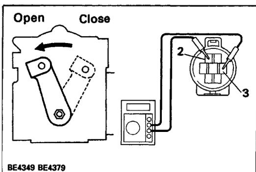
(b) When the arm is moving from the closed to open position, check that resistance between terminals 2 and 3 increases from approx. 0.5 to 1.7 k $\Omega$ .
