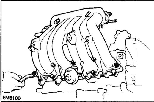
(c) Remove the four bolts, three nuts, intake manifold, T-VIS VSV and two gaskets.
