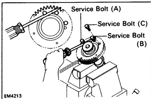
(d) Insert service bolts (A) and (B) into the service hole of the camshaft sub-gear.
