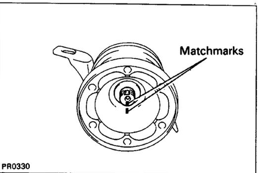
(c) Place the matchmarks on the rear flange and shaft.
