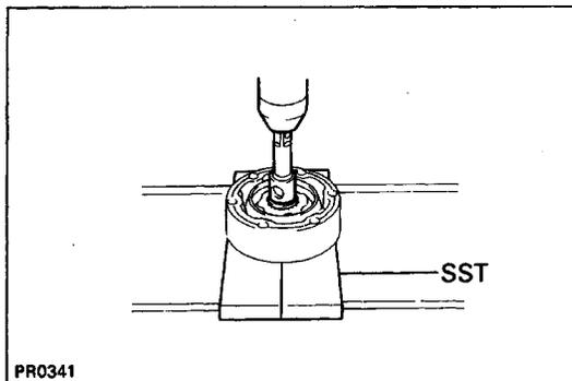
(e) Using SST, extension bar and press, remove the cross groove joint.
