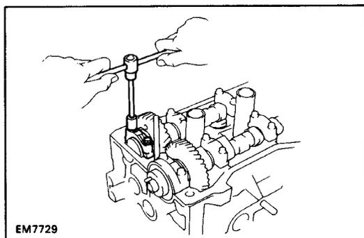
(b) Remove the two bolts and front bearing cap.
