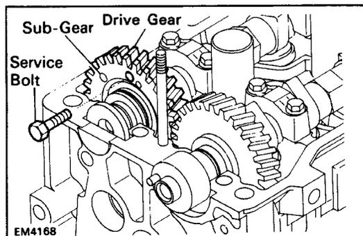
(c) Secure the intake camshaft sub-gear to the drive gear with a service bolt.
