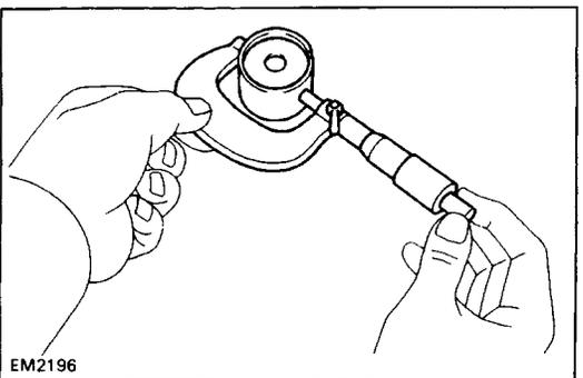
(b) Using a micrometer, measure the lifter diameter.
