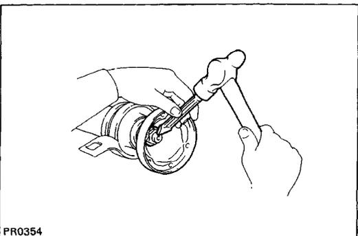
(g) Using a hammer and chisel, stake the nut.
