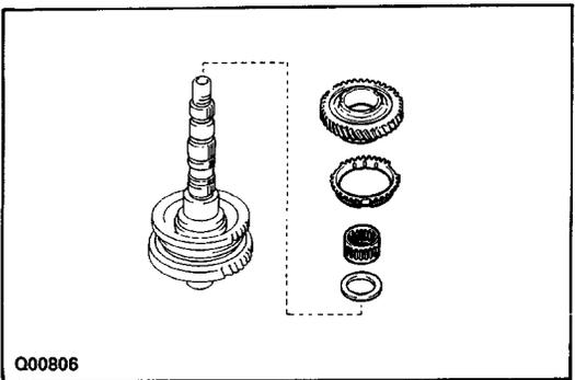
**6. INSTALL SYNCHRONIZER RING, SPACER, NEEDLE ROLLER BEARING, SECOND GEAR AND THIRD DRIVEN GEAR**
