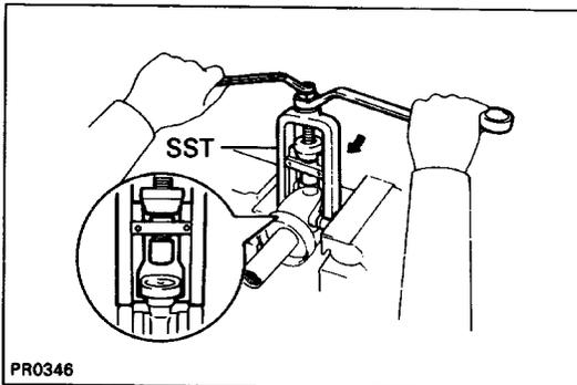
(c) Install the two removed bearing outer races to the spider.
