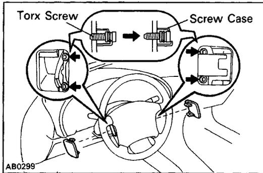
(e) Install the wheel pad after confirming that the circumference groove of the torx screws is caught on the screw case.
