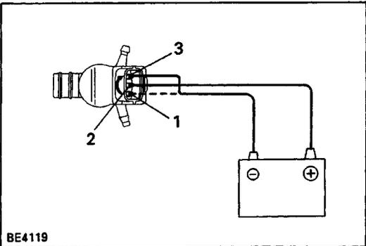
(b) Disconnect the negative (-) lead from terminal 1, and connect the negative (-) lead from the battery to terminal 3, check that the motor operates.
