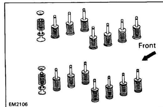
HINT: Arrange the valves, valve springs, spring seat: and spring retainers in correct order.
