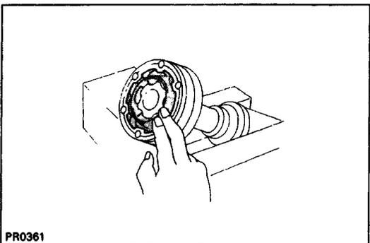
(f) Fill the grease into the joint.
