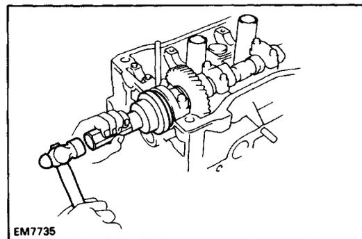
(i) Using SST, tap in the oil seal.
