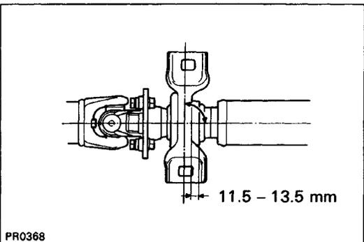
(c) Check that the center line of the bracket is at right angles at the shaft axial direction.
