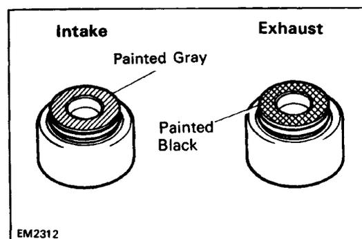
HINT: The intake valve oil seal is brown and the exhaust valve oil seal is black.
