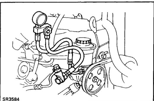
(b) Connect the gauge side of the pressure gauge to the PS pump and the valve side to the pressure line.
