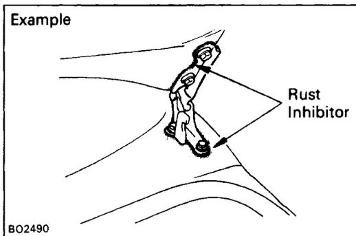
2. If a hinge or exterior body panel is loosened or removed, be sure to apply rust inhibitor after repairs.
