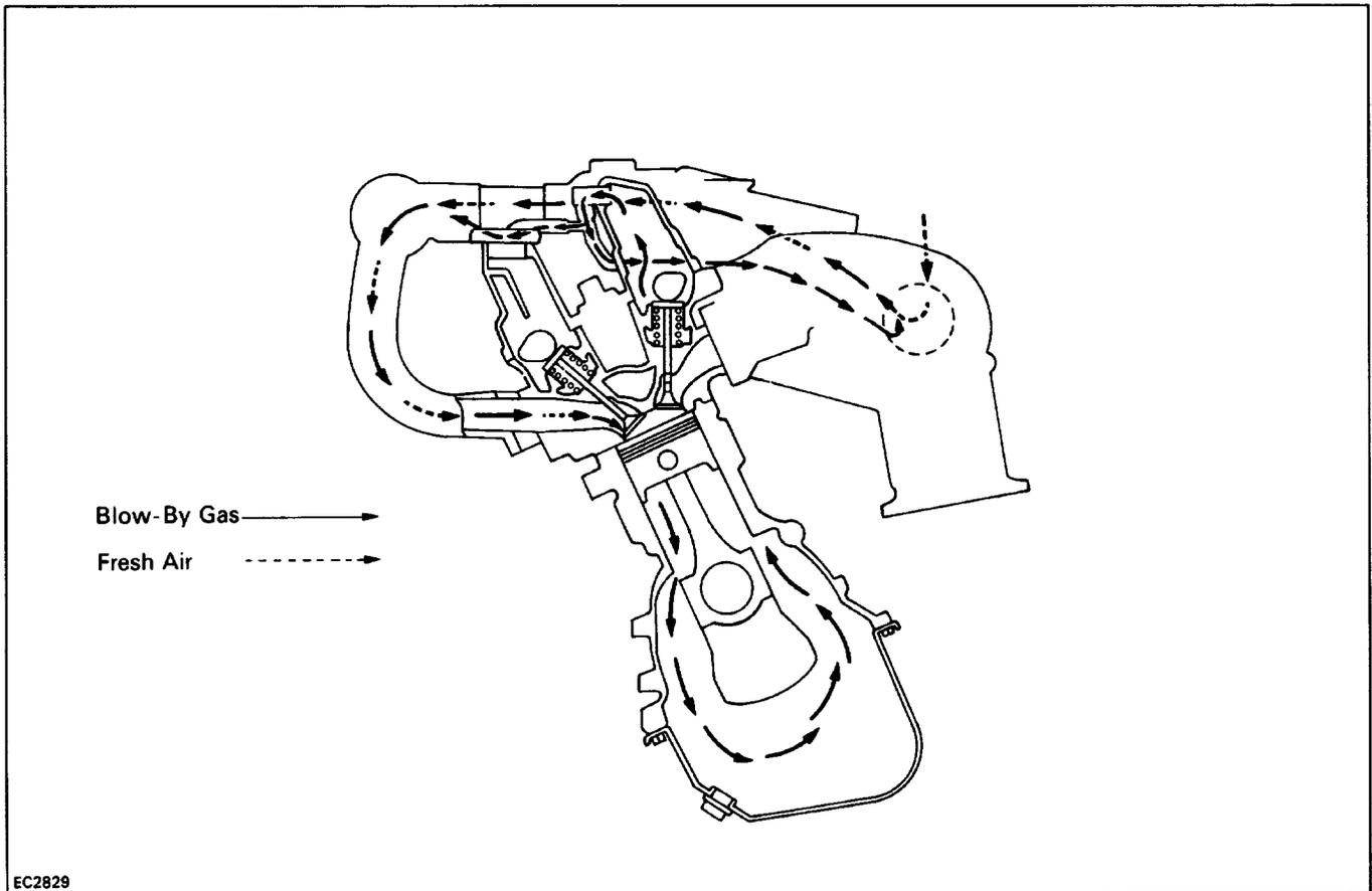
To reduce HC emissions, crankcase blow-by gas (HC) is routed to the intake manifold for combustion in the cylinders.
