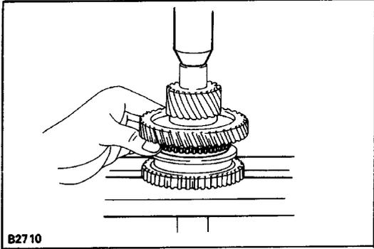
(f) Using a press, install the 1st gear and No. 1 hub sleeve.
