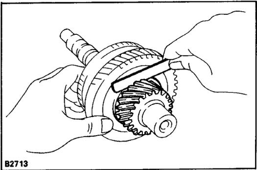
**5. INSPECT FIRST GEAR THRUST CLEARANCE**
