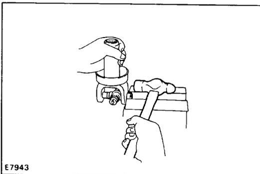
(e) Clamp the bearing outer race in a vise and tap off the yoke with a hammer.
