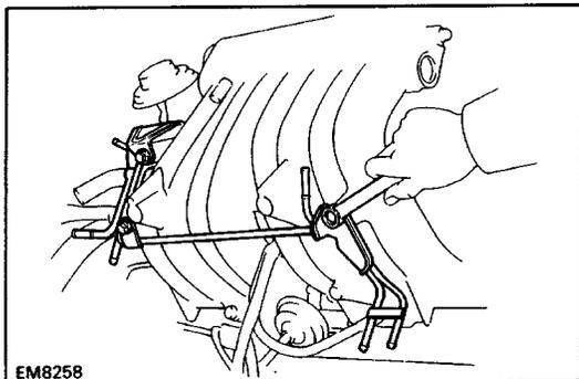
**29. REMOVE T-VIS VACUUM TANK, T-VIS VSV, TURBOCHARGING PRESSURE VSV AND BRACKET**
