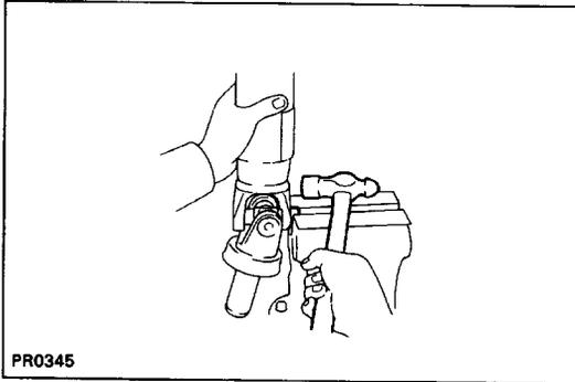
(b) Clamp the bearing outer race in a vise and tap off the shaft with a hammer.
