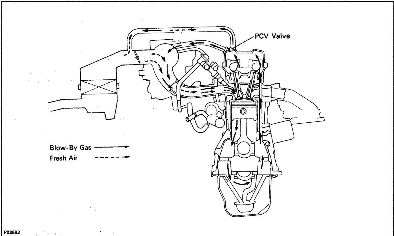
To reduce HC emissions, crankcase blow-by gas (HC) is routed through the PCV valve to the intake manifold for combustion in the cylinders.
