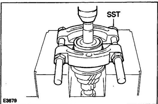
**4. REMOVE REAR BALL BEARING, FOURTH GEAR, NEEDLE ROLLER BEARING, SPACER AND SYNCHRONIZER RING FROM INPUT SHAFT**
