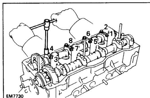
(d) Uniformly loosen and remove the eight bearing cap bolts in several passes in the sequence shown.
