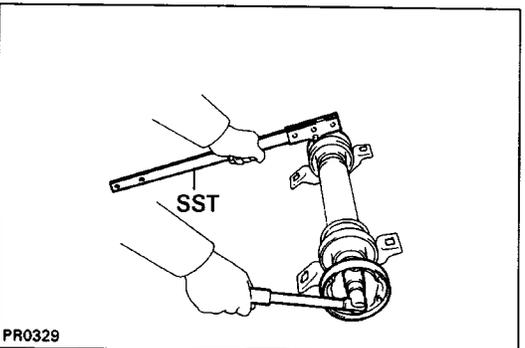
(b) Using SST to hold the front flange, remove the nut and plate washer.
