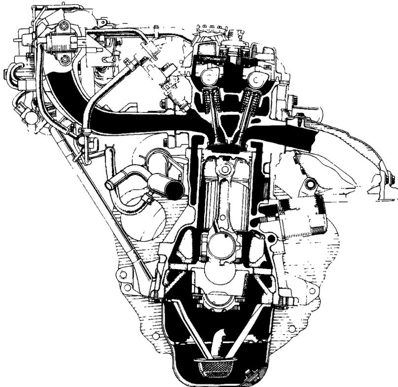
The 4A-FE engine is an in-line, 4-cylinder engine with the cylinders numbered 1 – 2 – 3 – 4 from the front. The crankshaft is supported by 5 bearings inside the crankcase. These bearings are made of aluminum alloy.
