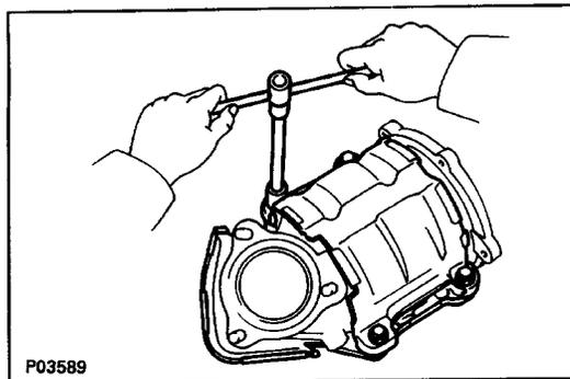
(d) Remove the five bolts and front heat insulator.
