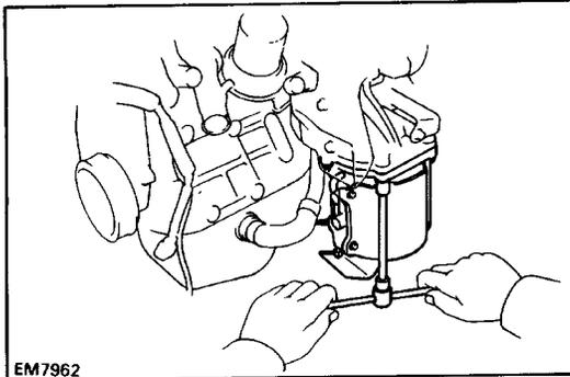
(e) Remove the three bolts, two nuts and three-way catalytic converter. Remove the gasket, retainer and cushion.
