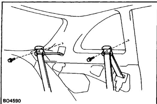
4. REMOVE FRONT SHOULDER BELT ANCHOR BOLT
