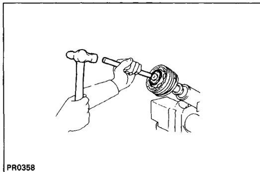
(b) Using a hammer and brass bar, tap the cross groove joint.
