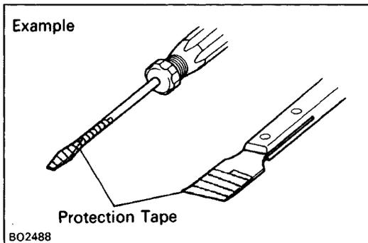
2. When prying off the body parts with a screwdriver or scraper, etc., be sure to apply protection tape to the tip or blade to prevent damage to the paint film or body part.
