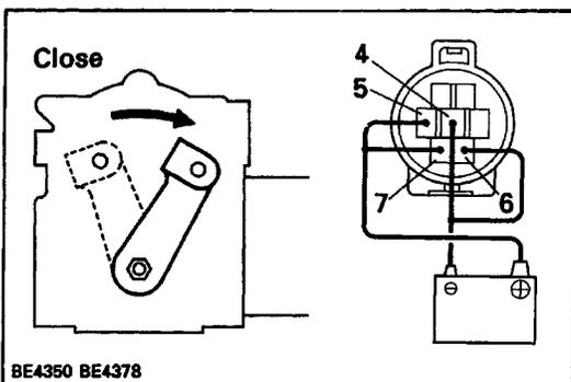
(c) With the magnet clutch ON, connect the positive (+) lead from the battery to terminal 7 and the negative (-) lead to terminal 6, check that the arm moves to the close side.
