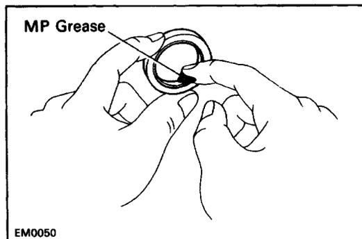
(h) Apply MP grease to a new oil seal lip.
