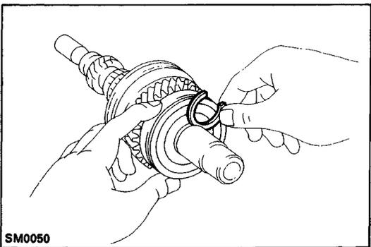
(b) Using a screwdriver and hammer, tap in the snap ring.
