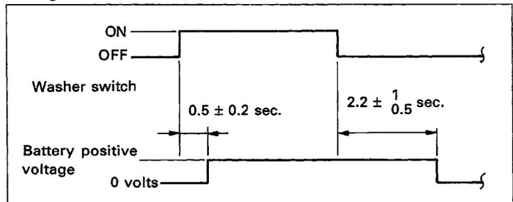
If operation is not as specified, replace the switch.
