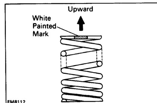
HINT: Install the valve spring, facing the white painted mark upward.
