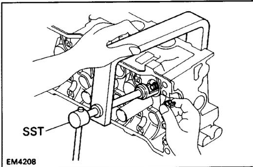
(c) Using SST, compress the valve spring and place the two keepers around the valve stem.
