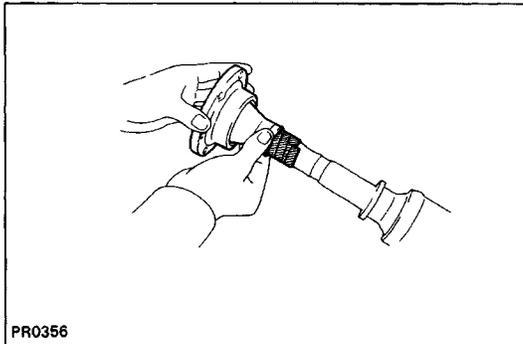
(b) Apply the adhesive tape from the top of shaft to the spline to prevent damaging the boot.
