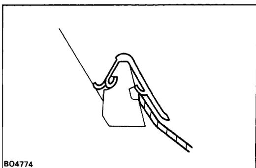
(b) Insert a scraper between the moulding and the body, then remove the moulding.
