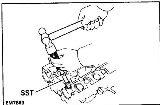
(c) Using SST and a hammer, tap out the guide bushing.
