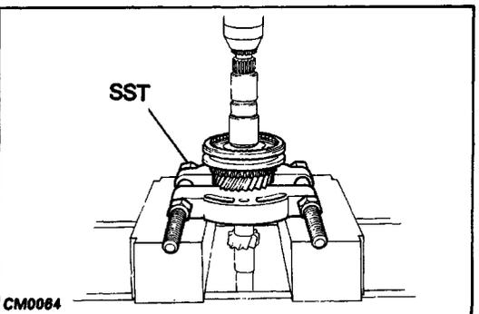
**6. REMOVE NO. 2 HUB SLEEVE ASSEMBLY, THIRD GEAR, SYNCHRONIZER RING AND NEEDLE ROLLER BEARING**
