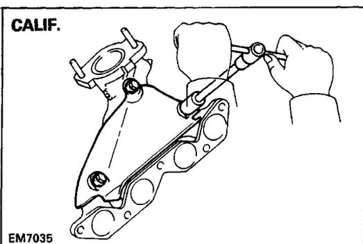
(d) Remove the three bolts and lower heat insulator from the exhaust manifold.
