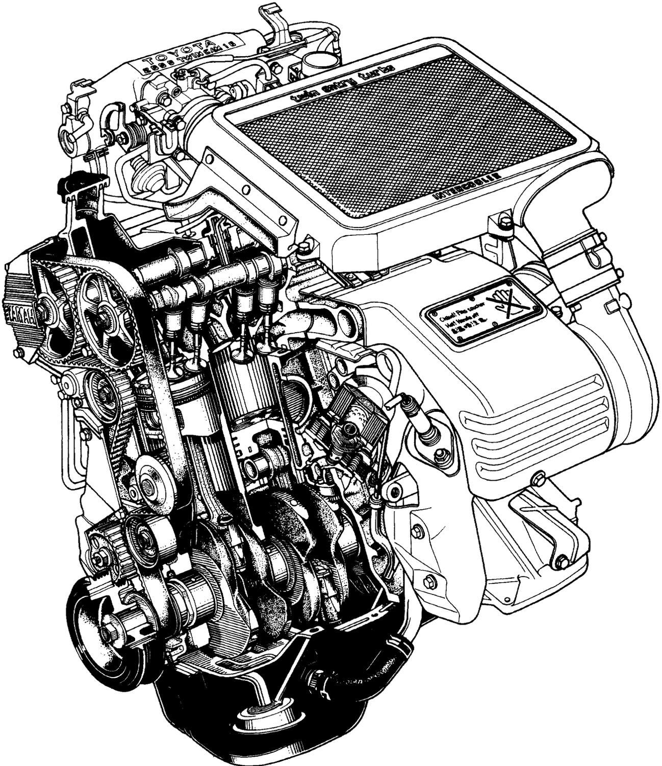
The 3S-GTE engine is an in-line, 4-cylinder engine with the cylinders numbered 1 – 2 – 3 – 4 from the front. The crankshaft is supported by 5 bearings inside the crankcase. These bearings are made of aluminum alloy.
