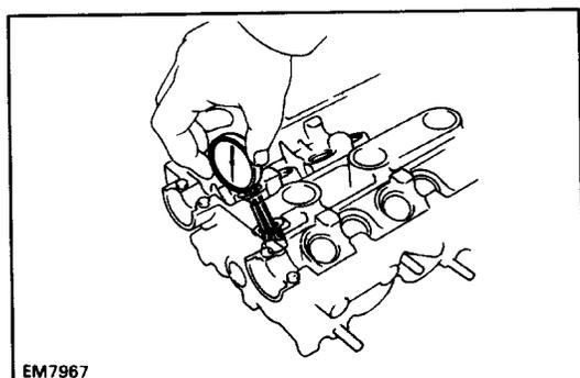
(d) Using a caliper gauge, measure the bushing bore diameter of the cylinder head.
