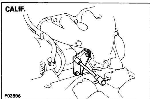
(b) Remove the three (CALIF.) or two (Ex. CALIF.) bolts and manifold stay.
