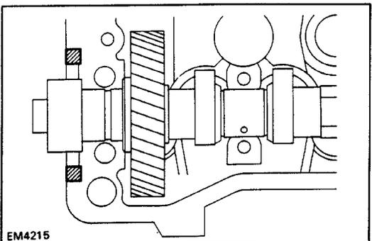
(c) Remove any old packing (FIPG) material.
