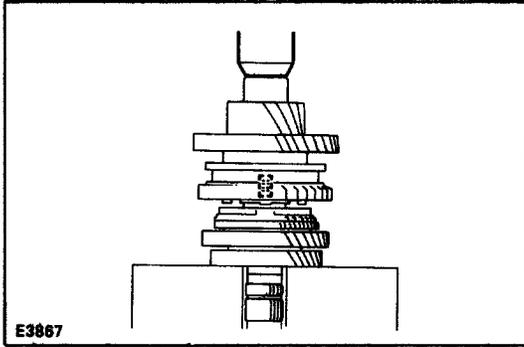
(e) Using a press, install the 3rd driven gear.
