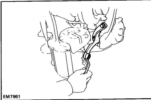
(b) Remove the three bolts and LH converter stay.
