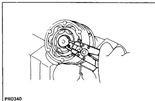
(c) Using snap ring pliers, install the new snap ring.
