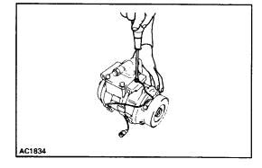
(c) Connect the stator lead wires to the compressor housing.
