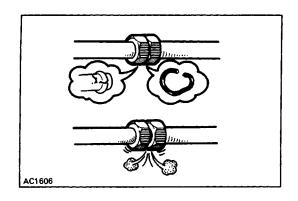
• Tighten the 4-ring fittings or the bolted type fittings to the specified torque.
