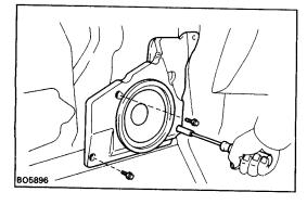
(g) (w/ Speaker)Connect the connector and install the speaker with three bolts.
