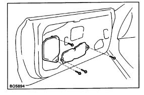
(e) Remove four screws, service hole cover No. 3 and No. 4.
