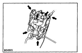
(b) Apply MP grease to the sliding surface of the door lock.
