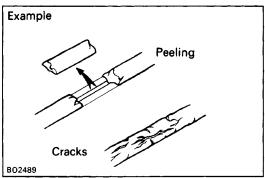
If anti-rust agents are damaged while repairing other parts, be sure to repair the anti-rust agent.
