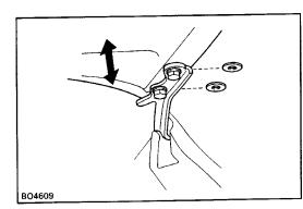
3. ADJUST REAR EDGE OF HOOD IN VERTICAL DIRECTION
