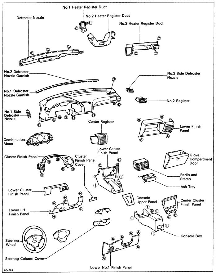
HINT: Screw sizes in the previous illustration are indicated by following the code below for removal and installation of safety pad.
