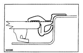
3. REMOVE WINDSHIELD MOULDING Using a knife, cut off the moulding as shown. NOTICE: Do not damage the body with the knife.
