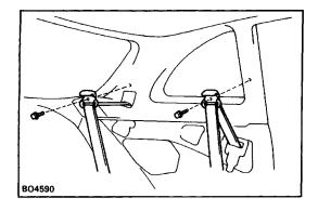
REMOVE FRONT SHOULDER BELT ANCHOR BOLT
