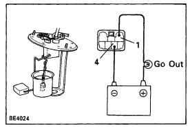
(b) Submerge the switch in fuel, check that the bulb goes
