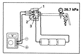
(e) Apply 26.7 kPa (200 mrnHg, 7.87 in.Hg) of vacuum. Check that the voltage drops below approximately 2.4 V.
