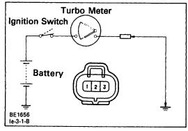
(c) Ground terminal 2 on the wire harness side. Check that the meter needle moves to lower position. If operation is not as specified, inspect the turbo meter drive circuit and resistance.
