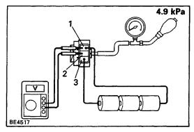
(f) Using SST, apply 4.9 kPa 10.5 kgf/cm<sup>2</sup>, 7.1 psi of pressure.
