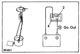
(b) Submerge the switch in fuel, check that the bulb goes out.
