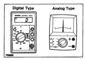
(c) Use a volt/ohmmeter with high impedance 110 k/V minimum) for troubleshooting of the electrical circuit.
