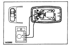
(c) Turn the room light switch DOOR, check that there is continuity between terminal 1 and 2.
