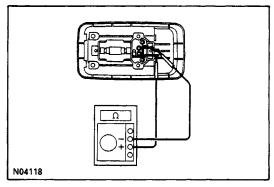
(c) Turn the room light switch DOOR, check that there is continuity between terminal 1 and 2.If operation is not as specified, replace the switch.
