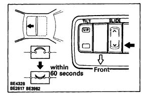
(b) With the sliding roof in fully opened position, hold the sliding roof switch in "CLOSE" position and check that the sliding roof begins to close within 60 seconds.If operation is not as specified, replace the motor.
