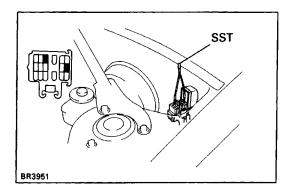
(e) Remove the SST from terminals Te and E1 of the data link connector 1. SST 09843–18020
