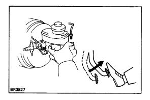
(c) Block off the outlet plug with your finger and release the brake pedal.
