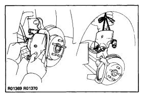
(b) Remove the brake cylinder and suspend it so the hose is not stretched.
