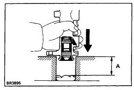
(c) Place a rag and two wooden blocks on the work table and lightly tap the cylinder flange against the block edges until the piston drops out of the cylinder.
