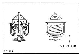
(c) Check the valve lift.
