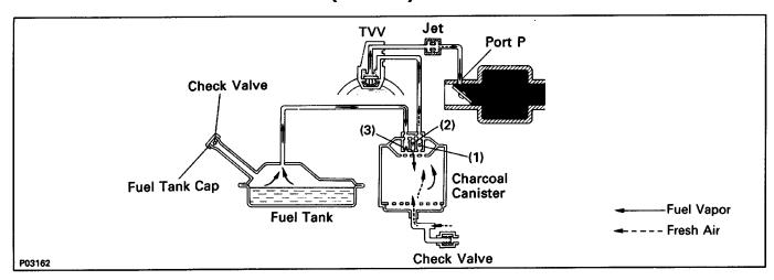
To reduce HC emissions, evaporated fuel from the fuel tank is routed through the charcoal canister to the intake manifold for combustion in the cylinders.
