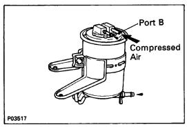
(b) Blow into port B and check that air does not flow from the other ports.
