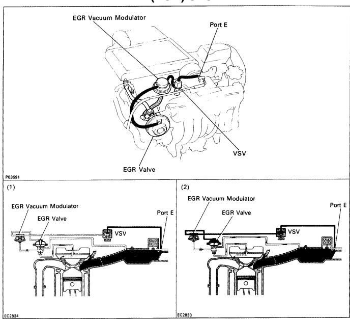
To reduce NOx emissions, part of the exhaust gases are recirculated through the EGR valve to the intake manifold to lower the maximum combustion temperature.
