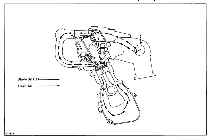
To reduce HC emissions, crankcase blow-by gas (HC) is routed to the intake manifold for combustion in the cylinders.
