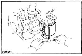
(c) Install the three–way catalytic converter with the three bolts and two new nuts.
