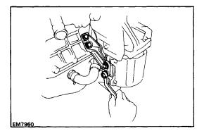
(d) Install the RH three–way catalytic converter stay with the four bolts.
