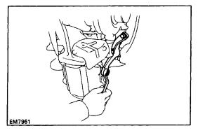
(c) Remove the three bolts and LH three-way catalytic converter stay.
