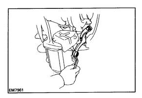
(e) Install the LH three–way catalytic converter stay with the three bolts.
