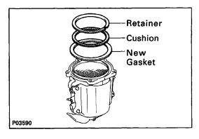
(b) Place the cushion, retainer and a new gasket or the three–way catalytic converter.
