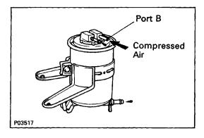
(b) Blow into port B and check that air does not flow from the other ports. If a problem is found, replace the charcoal canister.
