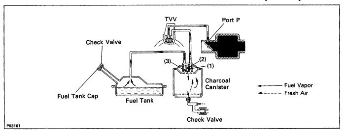
To reduce HC emission, evaporated fuel from the fuel tank is routed through the charcoal canister to the intake manifold for combustion in the cylinders.
