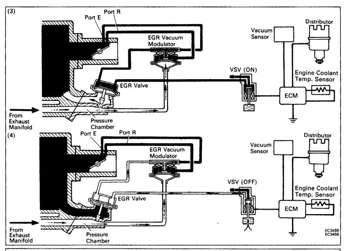
To reduce NOx emissions, part of the exhaust gases are recirculated through the EGR valve to the intake manifold to lower the maximum combustion temperature.
