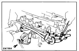
(b) Remove the two bolts, two nuts, water by–pass pipe, gasket and 0–ring.
