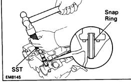
(g) Using SST and a hammer, tap in a new guide bush ing until the snap ring makes contact with the cylinder head.
