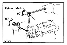
(d) Mark the front of the cylinder head bolt head with paint.
