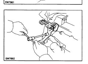
30. INSTALL NO.1 GENERATOR BRACKET AND RH FRONT ENGINE HANGER
