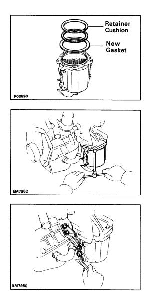
(c) Place a new gasket, the cushion and retainer on the three–way catalytic converter.
