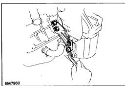
11. REMOVE THREE–WAY CATALYTIC CONVERTER(a) Remove the four bolts and RH converter stay.
