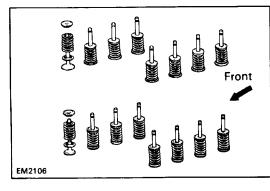
HINT: Arrange the valves, valve springs, spring seat: and spring retainers in correct order.
