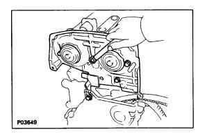
4. INSTALL NO-3 TIMING BELT COVER Install the N o.3 belt cover with the five bolts. Torque: 8.8 N-m (90 kgf-cm, 78 in.lbf)
