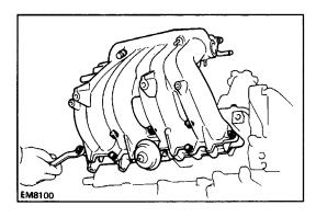
(c) Remove the four bolts, three nuts, intake manifold, T–VIS VSV and two gaskets.
