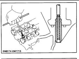
(h) Using a sharp 6 mm reamer, ream the guide bushing to obtain the standard specified clearance (See page EM-1 29) between the guide bushing and valve stem.
