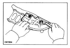
(b) Remove the bolt, nut and heat insulator. **16. REMOVE DISTRIBUTOR (See page IG-26)**
