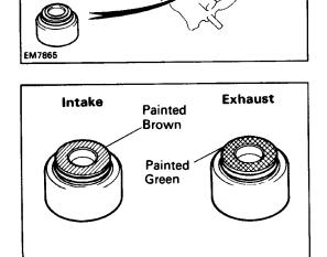
HINT: The intake valve oil seal is brown and the exhaust valve oil seal is black.
