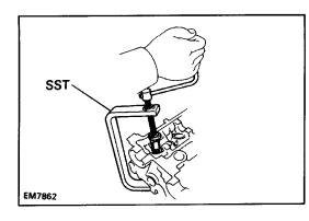
(c) Using SST, compress the valve spring and place the two keepers around the valve stem.
