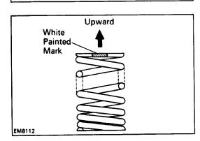
HINT: Install the valve spring, facing the white painted mark upward.
