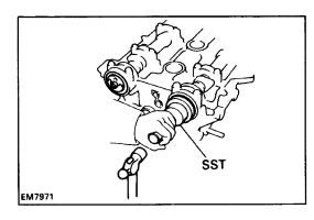
(g) Using SST, tap in the two camshaft oil seals. SST 09223–50010
