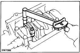
(h) Install the connecting rod cap.
