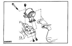
(b) Remove the through bolt, three bolts and LH mounting insulator.
