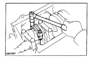
(i) Remove the connecting rod cap. (See procedure (b) and (c) above)
