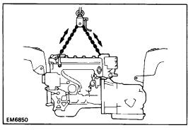
(c) Keep the engine level, and align RH and LH mountings with the body bracket.
