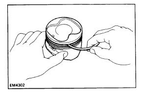
(b) Using a groove cleaning tool or broken ring, clear the piston ring grooves.
