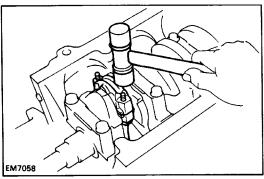
(c) Using a plastic–faced hammer, lightly tap the connecting rod bolts and lift off the connecting rod cap
