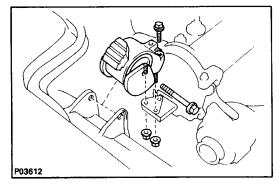
(d) Remove the through bolt, two nuts and RH mounting insulator.
