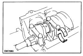
(e) Clean the crank pin and bearing.
