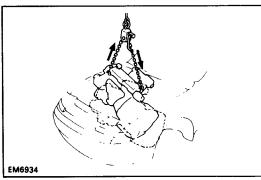
(e) Lift the engine out of the vehicle slowly and care—fully.
