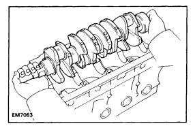
(c) Lift out the crankshaft.
