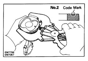
(b) Using a piston ring expander, install the two compression rings with the code mark facing upward (No.2 compression ring only).
