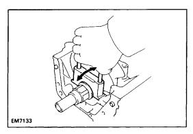
(b) Using the removed main bearing cap bolts, pry the main bearing cap back and forth, and remove the main bearing caps, lower bearings and lower thrust washers (No.3 main bearing cap only). HINT:
