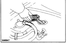
(b) Remove the two nuts, and pull out the engine wire from the cowl panel.
