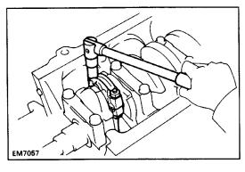
(b) Remove the connecting rod cap nuts.
