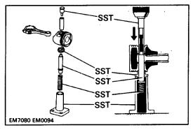
(c) Using SST, press in the piston pin. SST 09221-25024 (09221-00020, 09221-00030, 09221-00050,09221-00130,09221-00140)
