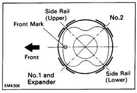
(c) Position the piston rings so that the ring ends are as shown.
