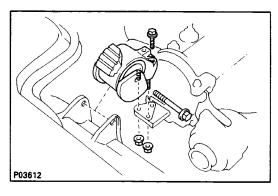
(d) Attach the RH mounting insulator to the mounting bracket and body, and temporarily install the through bolt and two nuts.
