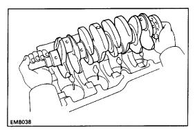
(c) Lift out the crankshaft.
