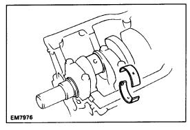
(e) Clean the crank pin and bearing.
