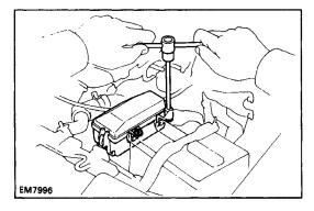
(c) Install the relay box with the two nuts.
