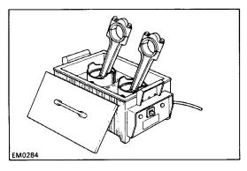
(b) Gradually heat the piston to  $80-90^{\circ}$ C (176–194°F).
