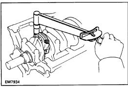
(h) Install the connecting rod cap.
