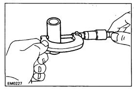
(b) Using a micrometer, measure the piston pin diameter.
