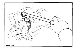
(i) Remove the connecting rod cap. (See procedures (b) and (c) above)
