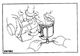
(c) Remove the three bolts, two nuts, three–way catalytic converter, cushion, retainer and gasket.
