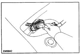
(b) Remove the two nuts, and pull out the engine wire from the cowl panel.
