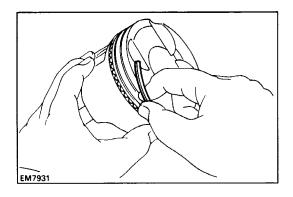
(b) Remove the two side rails and oil ring expander by hand.
