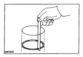
(c) Using a feeler gauge, measure the end gap.
