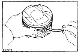
(b) Using a groove cleaner tool or broken ring, clean the piston ring grooves.
