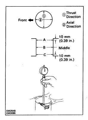
Using a cylinder gauge, measure the cylinder bore diameter at positions A,6 and C in the thrust and axial directions.
