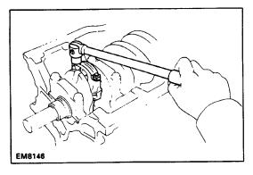
(b) Remove the connecting rod cap nuts.
