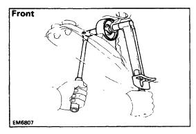
(b) Tighten the front through bolt.
