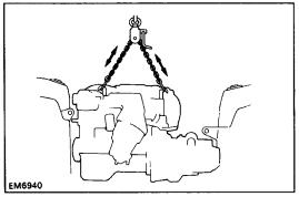
(c) Keep the engine level, and align RH and LH mountings with the body bracket.
