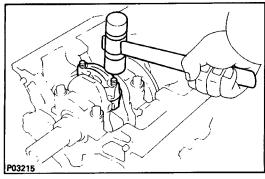
(c) Using a plastic–faced hammer, lightly tap the connecting rod bolts and lift off the connecting rod cap.HINT: Keep the lower bearing inserted with the connecting cap.
