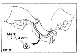
(b) Align the bearing claw with the claw groove of the main bearing cap, and push in the five lower bearings.
