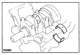
(e) Clean the crank pin and bearing.
