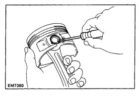
(e) Using a small screwdriver, install a new snap ring on the other side of the piston pin hole.
