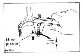
(b) If the cap nut cannot be turned easily, measure the outside diameter of the connecting rod bolt with a vernier caliper.
