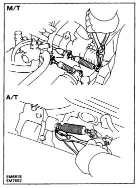
20. CONNECT TRANSAXLE CONTROL CABLE(S) TO TRANSAXLE.
