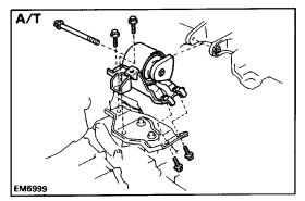
(f) Attach the LH mounting insulator to the mounting bracket and body with the through bolt and four bolts. Torque the bolts.
