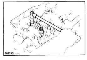
(b) Using SST, remove the connecting rod cap nuts. SST 09011–38121
