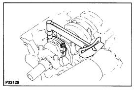
(h) Install the connecting rod cap.
