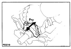
(b) Using the removed main bearing cap bolts, pry the main bearing cap back and forth, and remove the main bearing caps, lower bearings and lower thrust washers (No.3 main bearing cap only).
