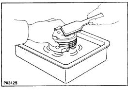
(c) Using solvent and a brush, thoroughly clean the piston.
