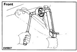
(b) Tighten the front through bolt.
