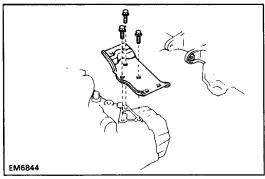
(e) Install the LH mounting bracket to the transaxle case with the three bolts.
