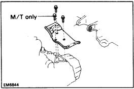
(c) Remove the three (M/T) or two (A/T) bolts and LH mounting bracket.
