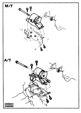
(b) Remove the through bolt, four bolts and LH mounting insulator.
