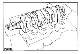
(c) Lift out the crankshaft.
