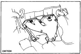
(c) Remove the two bolts, three nuts, exhaust manifold and gasket.
