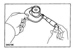
(b) Using a micrometer, measure the lifter diameter. Lifter diameter: 27.975 – 27.985 mm (1.1014 –1.1018 in.)
