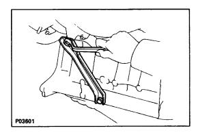
(c) Install the manifold stay with the two bolts. Alternately tighten the bolts.
