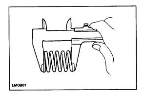
(b) Using a vernier caliper, measure the free length of the valve spring.
