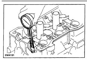
(c) Using a caliper gauge, measure the bushing bore diameter of the cylinder head.
