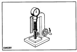
(c) Using a spring tester, measure the tension of the valve spring at the specified installed length.
