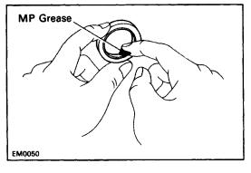
(h) Apply MP grease to a new oil seal lip.
