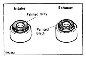
HINT: The intake valve oil seal is brown and the exhaust valve oil seal is black.
