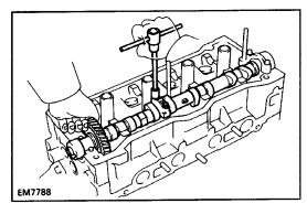
HINT: If the camshaft is not being lifted out straight and level, reinstall the No–3 bearing cap with the two bolts. Then alternately loosen and remove the two bearing cap bolts with the camshaft gear pulled up.
