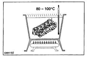
(e) Gradually heat the cylinder head to  $80 - 100^{\circ}$ C (1176  $-212^{\circ}$ F).
