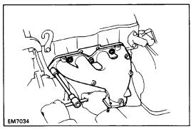
(c) Install the manifold stay with the three (CALIF.) or two (Ex. CALIF.) bolts. Alternately tighten the bolts.
