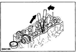
(f) Measure the Plastigage at its widest point. **Standard oil clearance:** 0.035 – 0.072 mm
