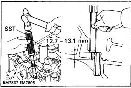
(f) Using SST and a hammer, tap in a new guide bushing until there is 12.7 –13.1 mm (0.500 – 0.516 in.) protruding from the cylinder head.
