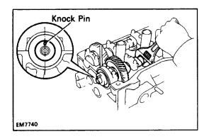
(1) Turn the exhaust camshaft clockwise, and set it with knock pin facing upward.
