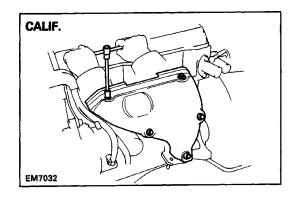
(d) Install the –upper heat insulator with the five (CALIF.) or four (Ex. CALIF.) bolts.
