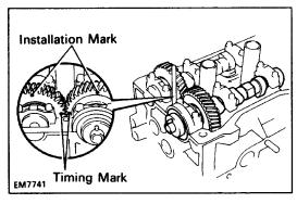
(m) Check that the timing marks of the camshaft gears are aligned.
