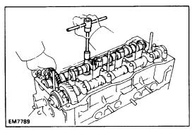
HINT: If the camshaft is not being lifted out straight and level, reinstall the bearing cap with the two bolts. Then alternately loosen and remove the bearing cap bolts with the camshaft gear pulled up.
