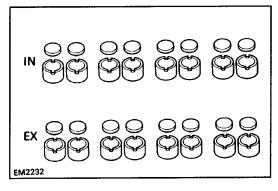
HINT: Arrange the valve lifters and shims in correct order.
