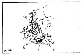
(b) Remove the two nuts, the vacuum pipe, vacuum modulator and VSV assembly.
