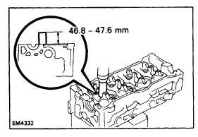
(b) Using a press, press in a new spark plug tube until there is 46.8 – 47.6 mm (1.843 –1.874 in.) protruding
