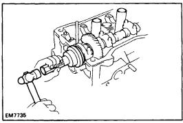
(i) Using SST, tap in the oil seal. SST 09223–46011
