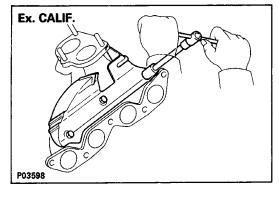
(b) Install a new gasket and the exhaust manifold with the two bolts and three new nuts. Uniformly tighten the bolts and nuts in several passes.
