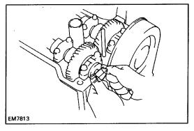
(c) Install the semi-circular plug to the cylinder head.
