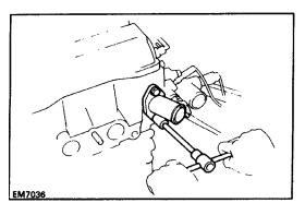
(c) Install the water inlet and inlet housing assembly with the bolt and two nuts.
