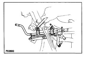
(b) Remove the two nuts and air pipe.
