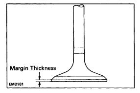
(c) Check the valve head margin thickness.
