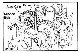
(c) Secure the intake camshaft sub-gear to the drivE gear with a service bolt.
