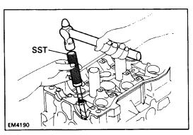
(b) Using SST and a hammer, tap out the guide bushing.
