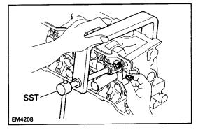
(c) Using SST, compress the valve spring and place the two keepers around the valve stem. SST 09202-70010
