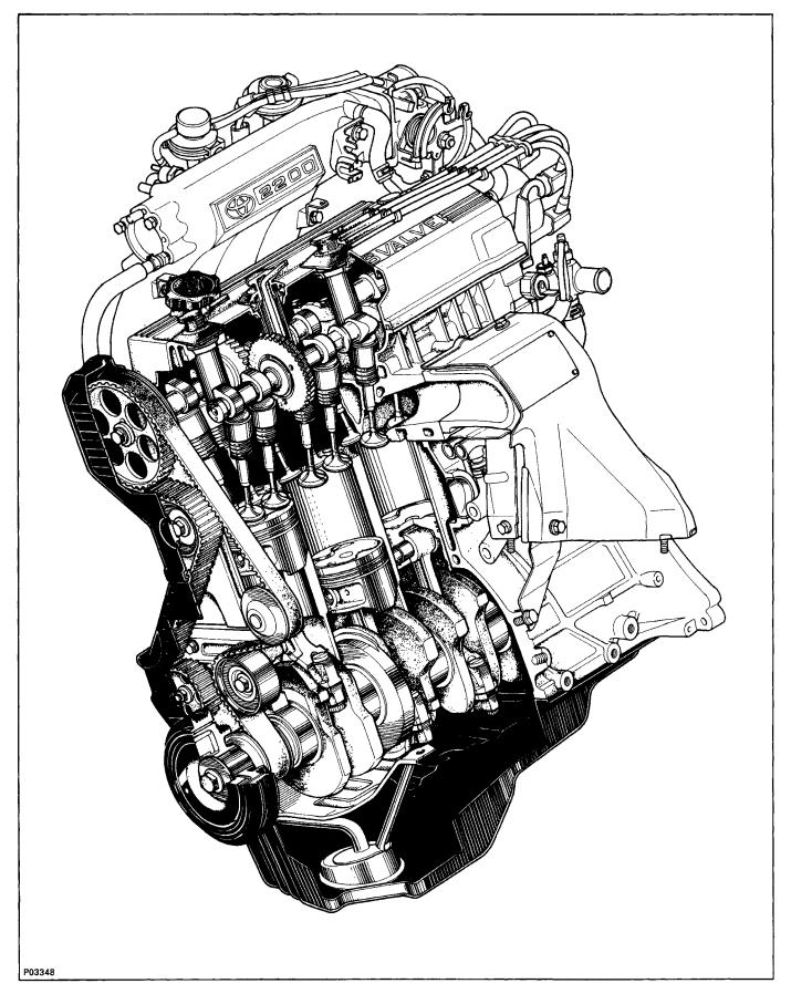
The 5S–FE engine is an in–line, 4–cylinder engine with the cylinders numbered 1 - 2 - 3 - 4 from the front. The crankshaft is supported by 5 bearings inside the crankcase. These bearings are made of aluminum
