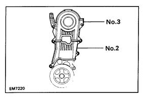
**13. REMOVE NO.3 AND NO.2 TIMING BELT COVERS** Remove the six bolts, engine wire bracket, No.3 and No.2 timing belt covers.
