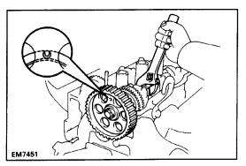
(b) Turn the hexagon wrench head portion of the camshaft, and align the hole of the camshaft timing pulley with the timing mark of the bearing cap. EM7341
