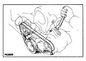
(b) Loosen the pivot nut and adjusting bolt, and remove the drive belt.
