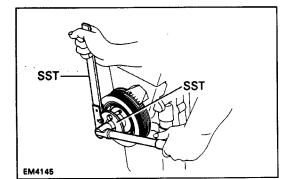
17. REMOVE CRANKSHAFT PULLEY (a) Using SST, remove the pulley bolt. SST 09213–14010 and 09330–00021
