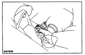
**19. INSTALL A/C IDLER PULLEY AND A/C DRIVE BELT** (a) Temporarily install the idler pulley with the nut.
