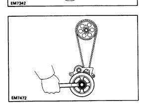
(b) Slowly turn the crankshaft pulley two revolution; from TDC to TDC.
