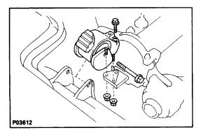
**15. INSTALL RH ENGINE MOUNTING INSULATOR** Install the mounting insulator with the through bolt, bolt and two nuts.
