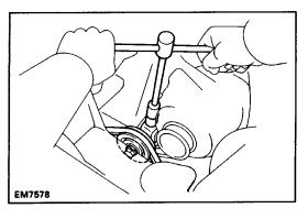
(b) Install the drive belt with the idler pulley nut and adjusting bolt.
