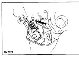
**21. REMOVE IDLER PULLEY AND TENSION SPRING** Remove the bolt, idler pulley and tension spring.
