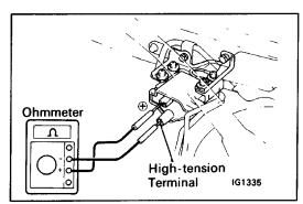
4. INSPECT SECONDARY COIL RESISTANCE Using an ohmmeter, measure the resistance between positive (+) and high–tension terminals.
