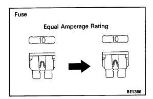
10. When replacing fuses, be sure the new fuse has the correct amperage rating. DO NOT exceed the rating or use one with a lower rating.
