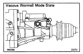
7. AFTER FINISHING TEST, BE SURE TO MOVE MODE SELECT LEVER BACK TO "VISCOUS (NORMAL) MODE" AND LOCK IT SECURELY WITH SET BOLT
