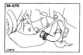
7. (3S–GTE) CONNECT TURBO OIL PIPE HOSE TO OIL PAN
