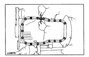
(c) Install the oil pan with the seventeen bolts and four nuts.
