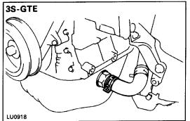
9. (3S-GTE) **DISCONNECT TURBO OIL PIPE HOSE FROM OIL-PAN**
