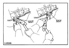
(c) Insert the blade of SST between the cylinder block and oil pan, cut off applied sealer and remove the oil pan.
