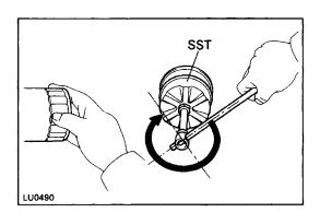
(e) Tighten the oil filter by hand until the rubber gasket contacts the seat of the filter mounting. Then using SST, give it an additional 3/4 turn to seat the oil filter.
