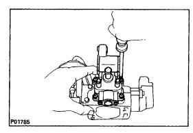
(b) Install the IAC valve with the four screws.
