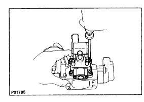
**2. REMOVE IAC VALVE** Remove the four screws, IAC valve and gasket.
