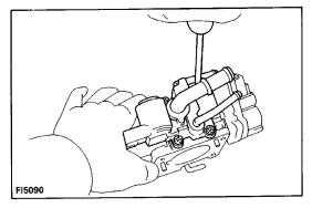
(b) Install the IAC valve with the four screws.
