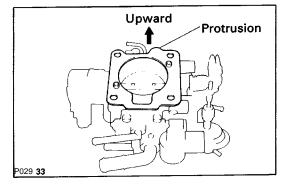
(b) Place a new gasket on the throttle body, facing the protrusion upward.
