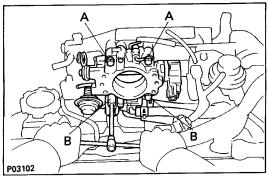
(c) Install the throttle body with the four bolts. **Torque: 19 N-m (195 kgf-cm, 14 ft-lbf)** HINT: Each bolt is indicated in the illustration. Bolt length: A 45 mm (1.77 in.)
