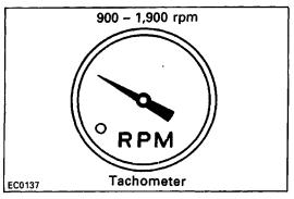
(b) Check the throttle opener setting speed.
