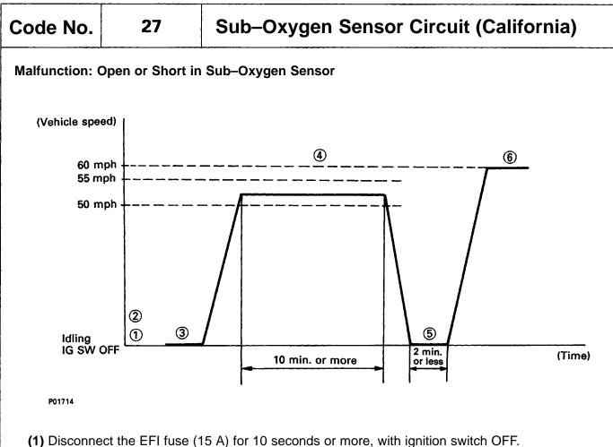
(2) Initiate test mode: Connect terminals TE2 and E1 of data link connector 1 with ignition switch OFF.
