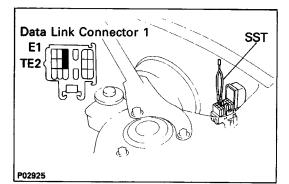
First, using SST, connect terminals TE2 and E1 of the data link connector 1, then turn the ignition switch on to begin the diagnosis in the test mode. SST 09843–18020
