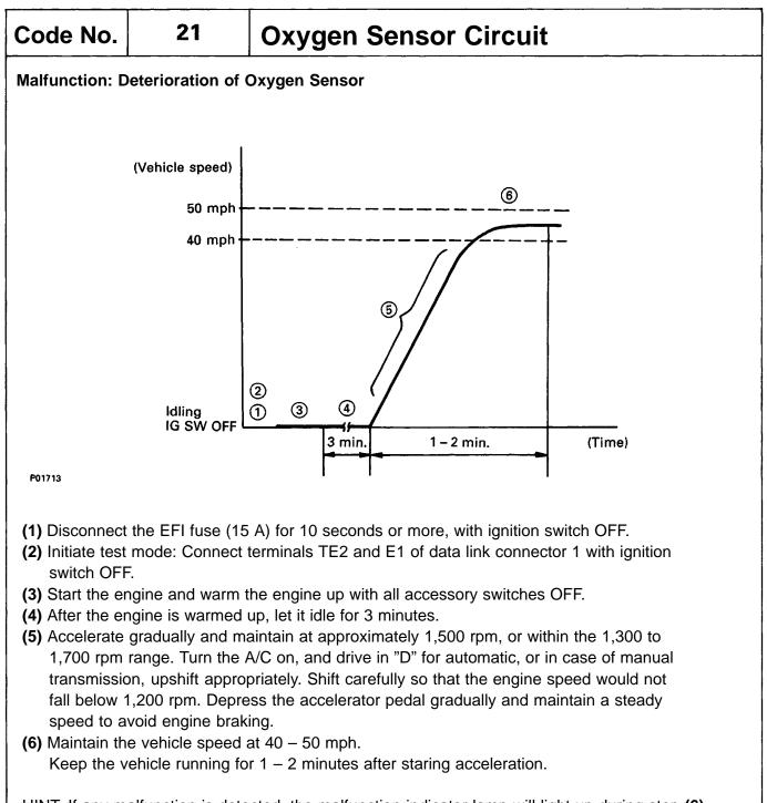
HINT: If any malfunction is detected, the malfunction indicator lamp will light up during step (6).
