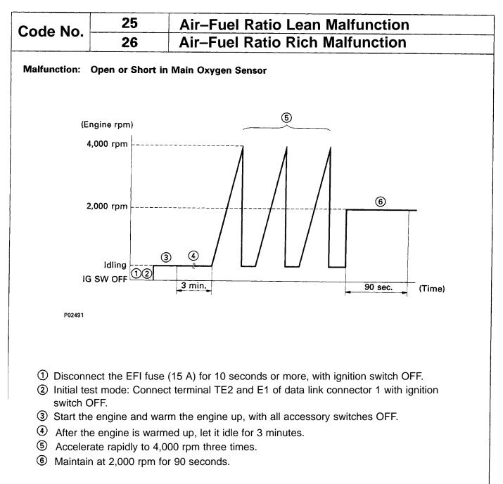
HINT: If a malfunction is detected, the malfunction indicator lamp will light up during step (6).
