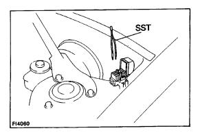
5. After the diagnostic check, remove the SST. SST 09843–18020
