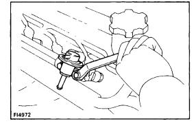
(b) Install the pressure regulator with the two bolts. Torque: 9.3 N-m (95 kgf-cm, 82 in.-lbf)
