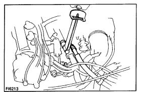
2. CONNECT FUEL INLET HOSE TO DELIVERY PIPE Connect the inlet hose with two new gaskets and the union bolt.
