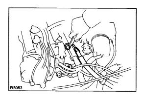
5. DISCONNECT FUEL INLET HOSE FROM DELIVERY PIPE Remove the union bolt and two gaskets, and disconnect the inlet hose from the delivery pipe.
