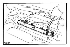
(h) Install the two bolts. Torque: 15 N–m (950 kgf–cm, 11 ft–lbf)
