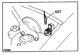
(c) When the fuel return hose is pinched, the pressure within high pressure line will rise to approx. 392 kPa (4 kgf/cm², 51 psi). In this state, check to see that there are no leaks from any part of the fuel system.
