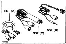
10. Use SST for inspection or test of the injector, cold start injector or its wiring connector.
