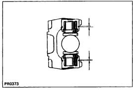
HINT: Adjust both bearings so that the snap ring grooves are at maximum and equal width.
