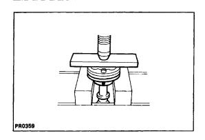
(d) Pass the bolt through to align the both bolt holes, then using a press and steel plate, press the universal joint cover with boot.
