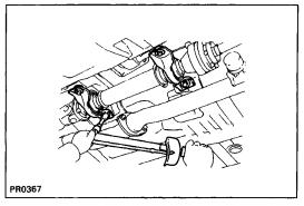
(b) With the same condition, adjust the intervals between the rear side of center bearing housing and the rear side of cushion at 11.5 – 13.5 mm (0.4528 in. – 0.5315 in.) as shown in the illustration below, then torque the bolts.
