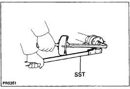
(d) Using SST to hold the flange, press the bearing into position by tightening down a new nut and washer. SST 09330-00021
