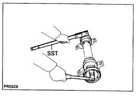
(b) Using SST to hold the front flange, remove the nut and plate washer.
