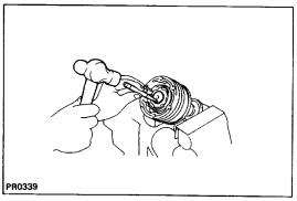
(c) Place the rnatchmarks on the inner race and shaft.
