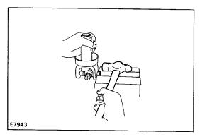
(e) Clamp the bearing outer race in a vise and tap off the yoke with a hammer.
