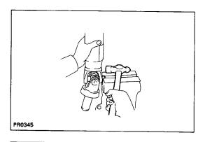
(b) Clamp the bearing outer race in a vise and tap off the shaft with a hammer.
