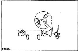
(b) Inspect the rear side of intermediate shaft flange runout in horizontal direction.
