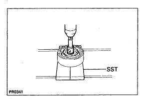
(e) Using SST, extension bar and press, remove the cross groove joint.
