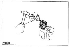
(b) Using a hammer and screwdriver, remove the cover.
