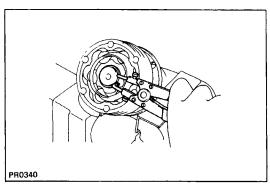
(c) Using snap ring pliers, install the new snap ring.
