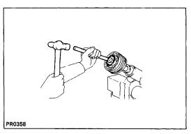
(b) Using a hammer and brass bar, tap the cross groove joint.
