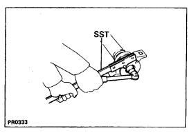
(b) Using SST to hold the flange, remove the nut and plate washer.
