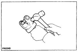
(b) Using a hammer, tap the yoke until there is no clearance between the bearing outer race and snap ring.
