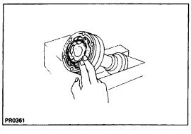
(f) Fill the grease into the joint.
