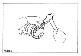
(g) Using a hammer and chisel, stake the nut.
