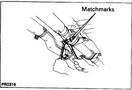
(c) Align the matchmarks on the both flanges, then install the bolts, washers and nuts.
