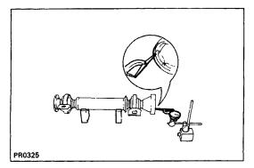
(c) Inspect the rear side of intermediate shaft flange runout in vertical direction.
