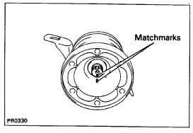
(c) Place the matchmarks on the rear flange and shaft.
