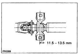
(c) Check that the center line of the bracket is at right angles at the shaft axial direction.
