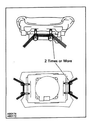
(1) Using 3 wire harnesses, wrap the wire harnesses at least 2 times each around the bolts installed on the left and right sides of the steering wheel pad.
