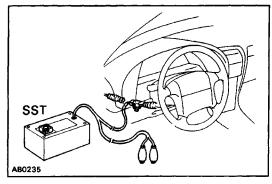
(c) Connect the SST connector to the airbag connector of the spiral cable.
