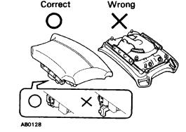
2. Never measure the resistance of the airbag squib. (This may cause the airbag to deploy, which is very dangerous.)
