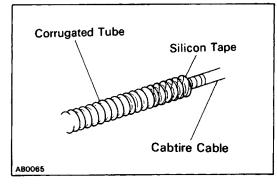
(f) Fix the corrugated tube to the cabtire cable using silicon tape.
