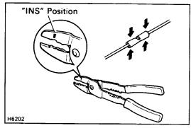
(f) Crimp both ends of the sleeve with the crimping too at the "INS" position.
