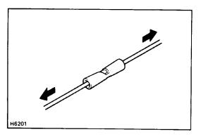
(e) Pull the joined wires to either end. Make sure that they are joined firmly by the sleeve.
