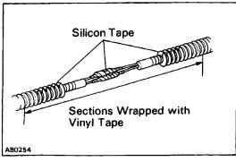
(g)After applying the silicon tape, apply vinyl tape on the corrugated tube of repair wire side over to the corrugated tube of vehicle wire harness side.
