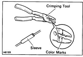
(c) The crimping tool (AMP Part No. 169060) has color marks on it. Place the sleeve in the correct section of the tool according to the color of the sleeve itself. HINT: As the crimping tool, AMP "Part No. 169060" is convenient to use.
