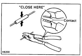
(d) With the center of the sleeve correctly placed between the crimping jaws, squeeze the crimping tool until either end comes into contact at the section marked by "CLOSE HERE".
