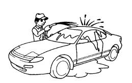
Sprinkle water onto the vehicle and check to see if the malfunction will occur.
