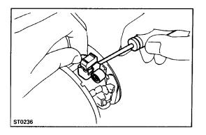
(c) Using a screwdriver, hold the spring back and dis– connect the brush from the brush holder. Discon– nect the four brushes, and remove the brush holder.
