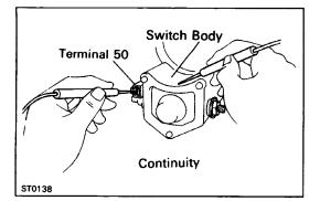
**2. PERFORM HOLD-IN COIL OPEN CIRCUIT TEST** Using an ohmmeter, check that there is continuity between terminal 50 and the switch body. If there is no continuity, replace the magnetic switch.
