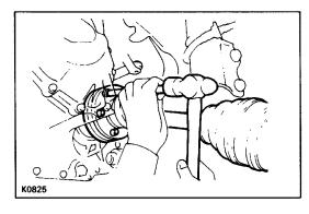
(c) Install the transmission case protector with two bolts.
