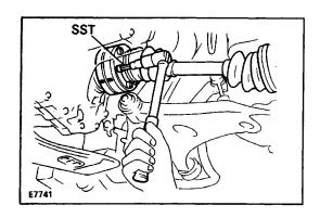
(e) Using SST, torque the six hexagon bolts while depressing the brake pedal.
