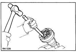
(b) Using a brass bar and hammer, tap the inboard joint onto the drive shaft.
