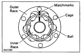
HINT: Should the joint become disassembled, reassemble it in the way shown.
