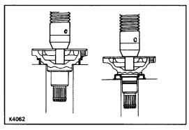
**11. INSTALL DUST COVER TO SIDE GEAR SHAFT** Using a press, install a new dust cover.
