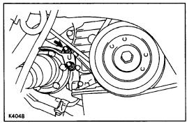
(d) Install the outboard joint side of the drive shaft to the axle hub.
