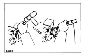
**9. REMOVE DUST COVER FROM SIDE GEAR SHAFT** Using a screwdriver and hammer, tap out the dust cover.
