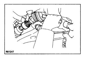
(g) Using a brass bar and hammer, drive out the drive shaft.
