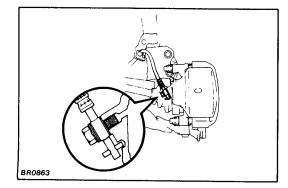
HINT: When connecting the brake hose to the caliper, connect so the peg aligns with the hole. (c) Install the clip.
