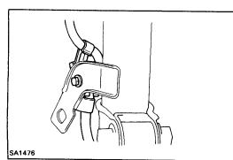
5. (w/ABS) CONNECT SPEED SENSOR WIRE HARNESS TO SHOCK ABSORBER
