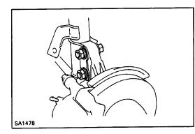
2. DISCONNECT SHOCK ABSORBER FROM STEERING KNUCKLE
